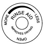
The clear indicator in the center of the cap changes from dark to light when the reservoir is nearly empty. This indicates that it is time to refill the dispenser.
